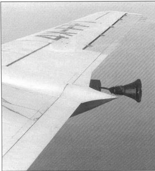
Left photo: This is the first ever published photo of the 4X-FPT that shows that this a/c served also as a refueling platform. Photo: Rami Skladman collection
