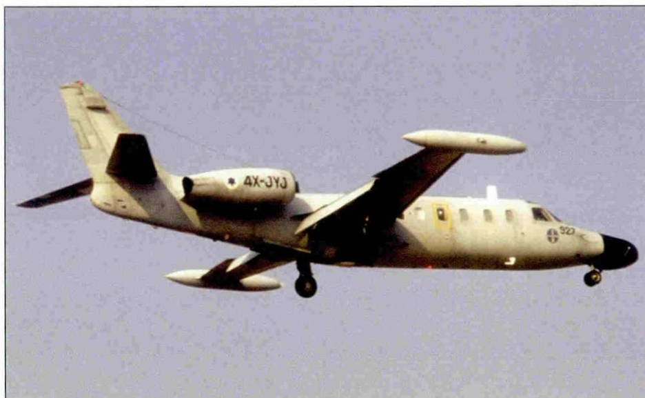
Left: A March 1975 PLO terrorist attack on the Savoy Hotel situated on the coast of Tel-Aviv pointed out the need for a long range shore patrol aircraft. Using surplus IAI model 1123 Westwind airframes it was decided upgrade them to model 1124 standards with the addition of a fuel saving Garret TFE731-3 turbopfan engines and a Litton model APS-504(V)2 marine search radar. Three Sea Scans were introduced into service with the International Transport squadron in 1979, serving alongside the Boeing 707 and wearing the same squadron insignia and colors on its motif. Sea Scans no.927 (4X-JYJ), no.929 (4X-JYR) and no.931 (4X-JYO) are currently painted in an overall RAL7023 Betongrau (~FS36280) Haze Grey finish with no identification features applied to the wings.
