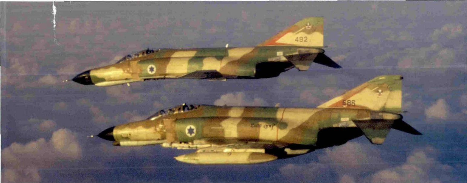
Top: Bat squadron Kurnass 2000 no.686 is seen in formation with HIAC camera nosed F-4E(S) no.492. Note the lack of wing and horizontal stabilizer low speed maneuvering leading edge slats and extended nose section of F-4E(S) no.492 in comparison to the Kurnass 2000 airframe.
