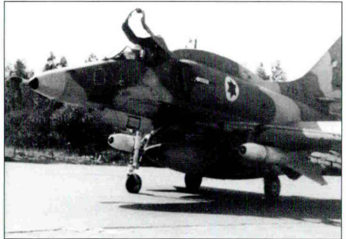
Above: This 1973 war photo shows Knights of the North squadron A-4E no.232 fitted with a pair of Walleye II optically guided bombs and an AIM-9B sidewinder on the outboard rail. In order to deliver these guided bombs, a telemetry pod was fitted on the opposite outboard pylon.
