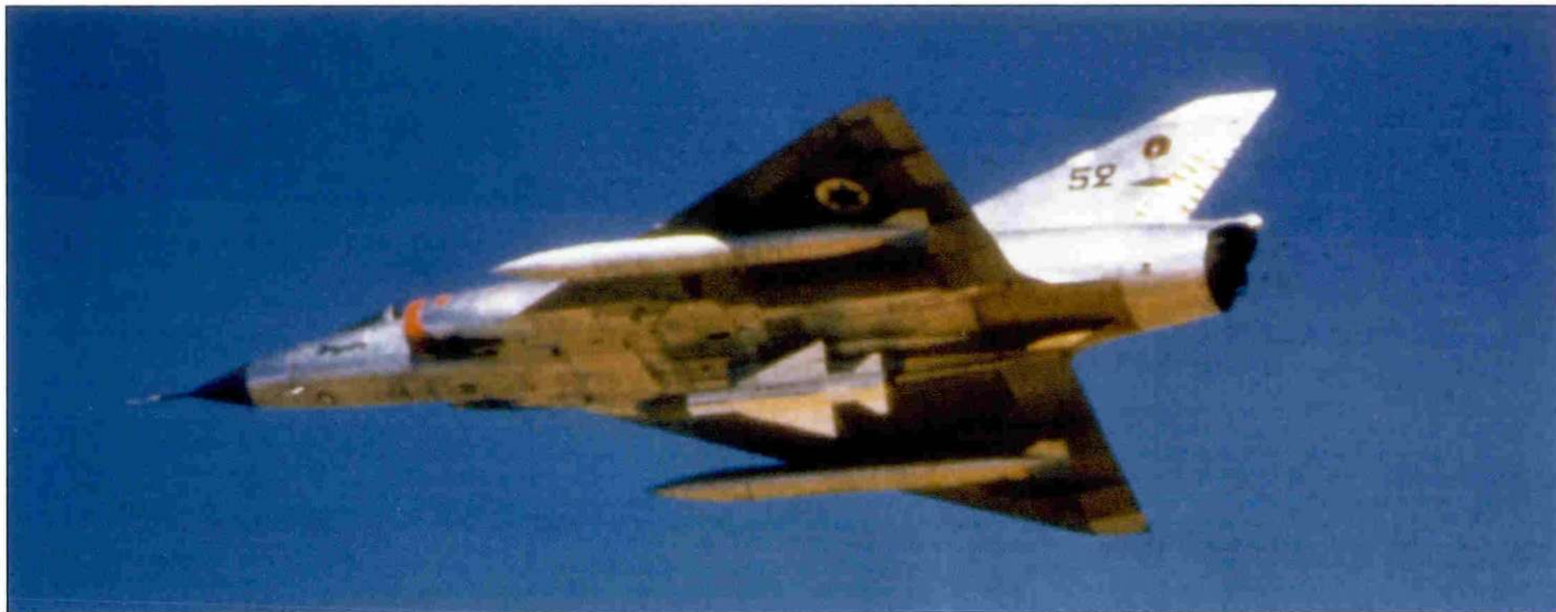
Above: Mirage IIIc no.52 of the First Fighter squadron is seen with a Matra 530 radar-guided air to air missile attached its centerline pylon. The Matra 530 was designed to down high altitude low maneuverable bombers such as the TU-16 and IL-28 in Arab service and proved useless in air combat against nimble MiG fighters. On November 29, 1966 the IAF attained its only Matra 530 kill (credited to Mirage no.52) when an unlucky Egyptian MiG-19 pilot broke into the flight path of the missile instead of away from it.
