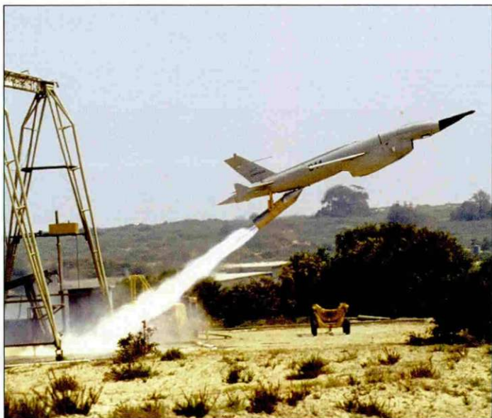
Left: Teledyne Ryan model 147T (AQM-34F) "Firebee" was first introduced into IAF inventory in July 1971. The long range, 60,000-ft. ceiling and 420 knot airspeed of the Firebee made it the ideal platform for high altitude reconnaissance over SAM threat areas. After several air engagements between Israel and Syria over Lebanon, Syria moved their SAM umbrella from along the border to inside Lebanon. Throughout the month of May 1981 IAF launched a large number of Firebee drone missions to monitor Syrian activities within Lebanon. The high-flying drones were easily detected by Syrian early warning radar and were often intercepted by Syrian MiG-21's. The poor turning rate of the Firebee made it easy pray for the MiG pilots but the lack of a pilot in the Firebee enabled new tactics to be developed using extremely high instantaneous turn rates such as steep climbs and steep dive to shake off the MiG pilots. On a mission that took place on May 14, 1981 a Syrian pilot in chase of an overall FS16440 Light Gull Grey Firebee, had to eject from his MiG-21 after entering a deep stall and losing control of his aircraft. Several days after the event, the IAF's first remotely piloted vehicle squadron was credited with the world's first kill for an unpiloted aircraft.
