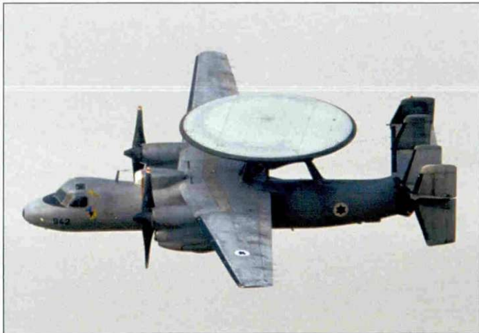
Left: Four Grumman E-2C Hawkeyes, named "Daya" by the IAF, entered service with the IAF during 1981 and were assigned identification numbers 941, 942, 944 and 946. The Hawkeye's ability to detect low flying aircraft through ground clutter and over water played a key roll in the IAF's ability to down 86 Syrian fighters in the first three days of the Lebanon War. These aircraft entered service in a Compass Ghost Grey color scheme of overall FS36375 Light Ghost Grey with FS36320 Dark Ghost Grey disruptive upper pattern camouflage.
