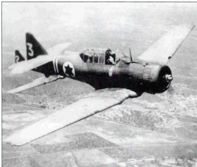
Above: AT-6 Texan no.1103 - In November 1948 the IAF introduced four digit identification numbers to its airplanes with the Texan & Harvard receiving 1100 series numbers. Since no roundels were specified for the upper wing surfaces, Texans converted dive-bombers had the last digit of their identification number applied atop of the wings and both sides of the rudder.
