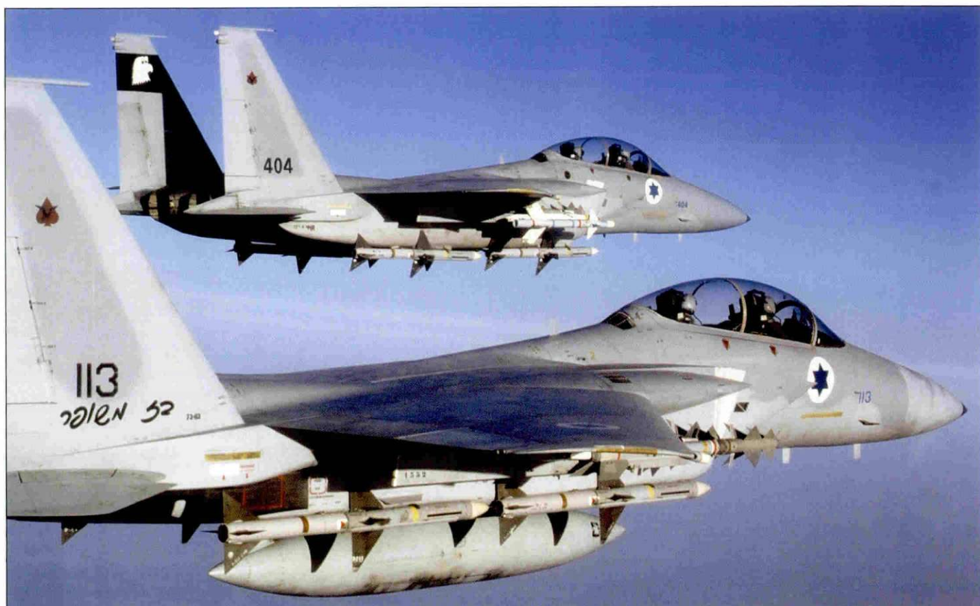
Above: First Eagle squadron F-15D no.404 and F-15B no.113 are seen in an air to air combat configuration. F-15D no.404 is fitted with a pair of Python IV on the inboard and Python III air to air missiles on the outboard pylons, and four AIM-7M Sparrow radar guided missiles. F-15B no.113 serial no.73-113 fitted with four Python IV's and four AIM-7M Sparrows. F-15B no.113 is one of 25 USANG surplus Eagles that were received as grant from the US after the 1991 Gulf War beginning on October 23, 1991. These Eagles were overhauled and upgraded to F-15D Improved Eagle standard beginning in 1998. The Hebrew inscription at the base of the vertical fin reads "Improved Eagle".
