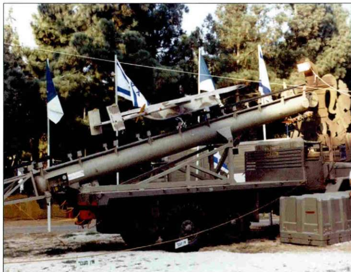
Left: Teledyne Ryan model 147T (AQM-34F) "Firebee" was first introduced into IAF inventory in July 1971. The long range, 60,000-ft. ceiling and 420 knot airspeed of the Firebee made it the ideal platform for high altitude reconnaissance over SAM threat areas. After several air engagements between Israel and Syria over Lebanon, Syria moved their SAM umbrella from along the border to inside Lebanon. Throughout the month of May 1981 IAF launched a large number of Firebee drone missions to monitor Syrian activities within Lebanon. The high-flying drones were easily detected by Syrian early warning radar and were often intercepted by Syrian MiG-21's. The poor turning rate of the Firebee made it easy pray for the MiG pilots but the lack of a pilot in the Firebee enabled new tactics to be developed using extremely high instantaneous turn rates such as steep climbs and steep dive to shake off the MiG pilots. On a mission that took place on May 14, 1981 a Syrian pilot in chase of an overall FS16440 Light Gull Grey Firebee, had to eject from his MiG-21 after entering a deep stall and losing control of his aircraft. Several days after the event, the IAF's first remotely piloted vehicle squadron was credited with the world's first kill for an unpiloted aircraft.
