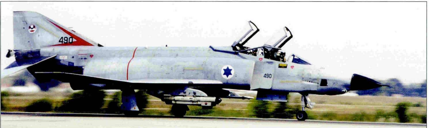
Above: RF-4E no.490 is one of six Peace Echo V Ghost Grey RF-4E's supplied to the IAF between 1976 and 1977. RF-4E no.490 is the only recognizance Phantom of the lot to retain its original external camera-opening configuration. Note the short ALQ-119 ECM pod on the right hand pilot and the missile rails on the left wing pylon used for carrying AIM-9L versions of the Sidewinder missile.
