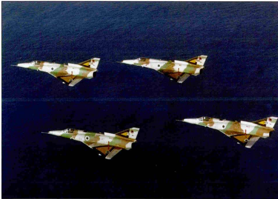
Above: Kfir no.709 - The first Israel Aircraft Industries Kfirs were transferred to the First Fighter squadron on April 14, 1975. Installation of the Phantom II's General Electric J79 engine offered the Mirage/Nesher airframe 30% greater thrust with 17% reduction in fuel consumption. This translated to greater weapons load capability and range than was possible in the aging Mirage and Nesher airplanes that were in IAF inventory.
