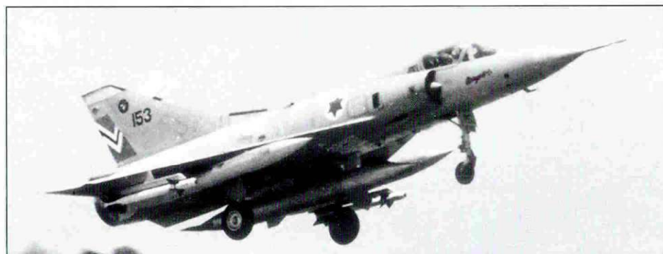
Left: Compass Ghost Grey camouflaged Mirage 153 is seen taking off in a rapid reaction alert intercept configuration with a 880 liter center line supersonic fuel tank, a pair of 500 liter supersonic wing tanks and a pair of Shafrir II IR homing air to air missiles. The Negev squadron operated the Mirage at the end of 1978 until they were replaced by F-16A/B Netz in September 1981.
