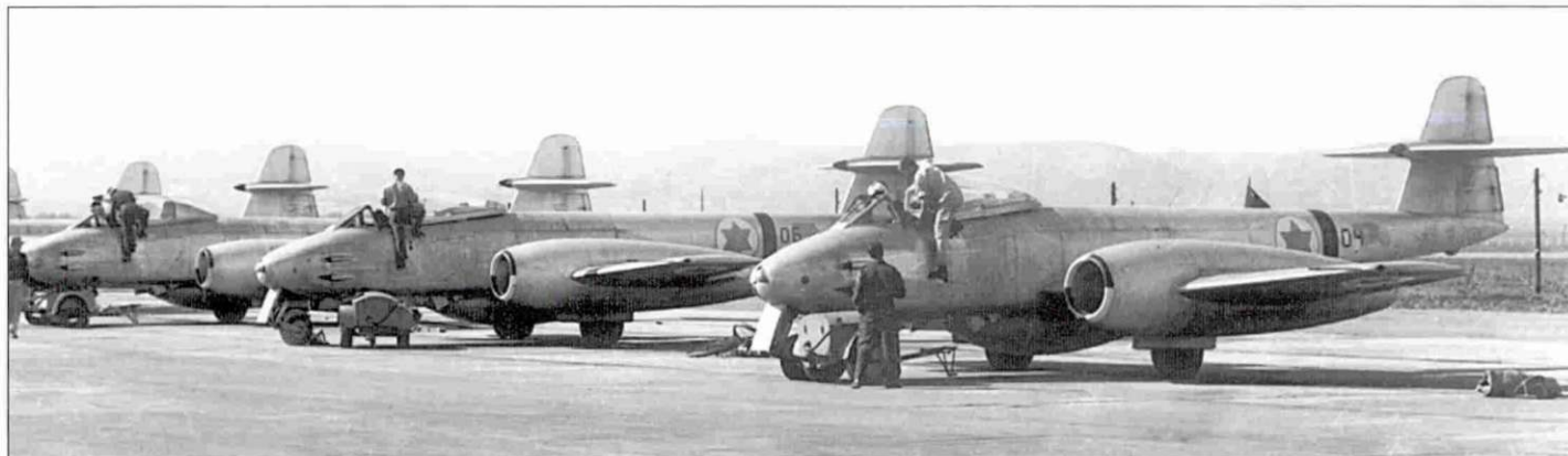
Above: A Suez War Meteor F.8 First Jet squadron line up with airplanes 04 and 06 in the foreground. Meteor 06 is seen with a black aft fuselage and wing identification bands applied where as Meteor 04 has only aft fuselage band applied. The wing bands were applied diagonally, starting at the wing leading edge outboard of the wing walkway boundaries and ending at the wing rear spar ahead of the ailerons. Additional Meteor F.8's seen with wing bands were 02 and 11.
