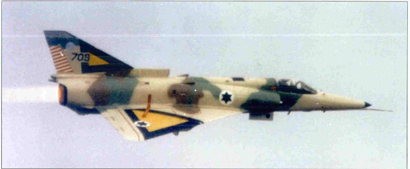
Above: Kfir no.709 - The first Israel Aircraft Industries Kfirs were transferred to the First Fighter squadron on April 14, 1975. Installation of the Phantom II's General Electric J79 engine offered the Mirage/Nesher airframe 30% greater thrust with 17% reduction in fuel consumption. This translated to greater weapons load capability and range than was possible in the aging Mirage and Nesher airplanes that were in IAF inventory.
