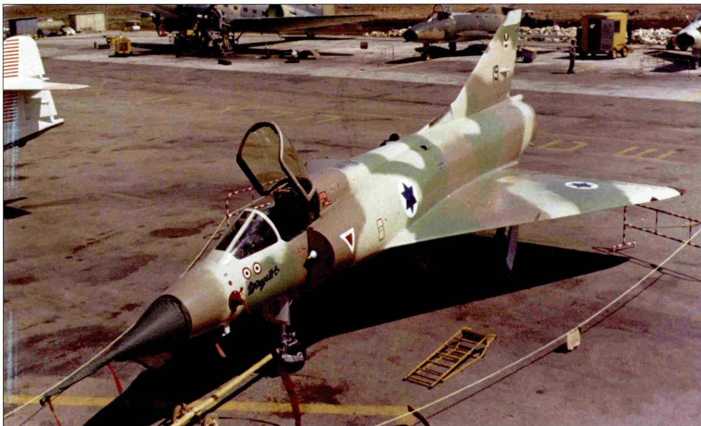
Above: Bat squadron Mirage IIIc no.19 is seen at IAI flight line after being painted in post-67 war colors of RAL1001 Beige (~FS33531 sand), RAL6011 Resedagrun (~FS34227 green), RAL8024 Beigebraun (~FS30219 tan) and RAL7035 Lichtgrau (~FS35662 light blue) undersurface. Egypt's introduction of the SAM-2 and SAM-3 high and medium altitude surface to air missiles along the Suez front during the July 1967 - August 1970 War of Attrition forced the IAF to fly a nap of the earth to avoid radar detection.
