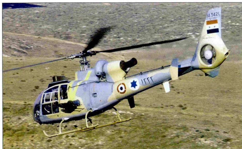
Left: Two Syrian Gazelles were found virtually intact after suffering minor battle damage that forced their abandonment in Lebanese territory. The two Gazelles were transported to Tel-Nof air base, where the 22 heavy maintenance unit joined parts from the two to make Gazelle no.1333 (s/n 1787) airworthy. Seventeen days after their arrival, Gazelle no.1333 made a flying appearance in the July 20, 1982 Israeli Air Force Day air display. The second Gazelle, no.1222 (s/n 659) was eventually restored as well and is currently on display at the IAF museum. Gazelle no.1333 shown here is painted using paints of local mix. The light tan color is a mixture of FS33531 sand and FS30219 tan at a ratio of 1:1. The green is FS34424 green to which 12% FS35090 blue is added. The undersurface color is FS36375 Light Ghost Grey with
