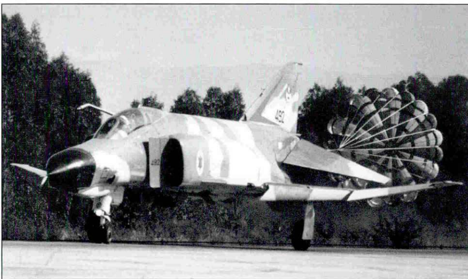
Above Left & Right: Between 1974 and 1976, three in service F-4E Phantoms were modified by General Dynamics to carry the oblique photography recognition camera known as HIAC. For this modification the nose section was extended by 12 inches and its Vulcan canon and radar were removed. F-4E serial numbers 69-7567, 69-7570 and 69-7576, designated as F-4E(S) after the modification, were returned to the IAF in 1976 and were given tail number 492, 498 and 499 by the Bat squadron. In 1980 during a mission over Iraq, a pair of HIAC equipped F-4E(S) were challenged by Iraqi MiG-21bis aircraft. While chasing F-4E(S) no.498 one of the MiG's ran out of fuel and the pilot jettisoned, leaving his aircraft to crash into the ground. For this "economical" kill, F-4E(S) was credited with a triangular Iraqi kill marking.
