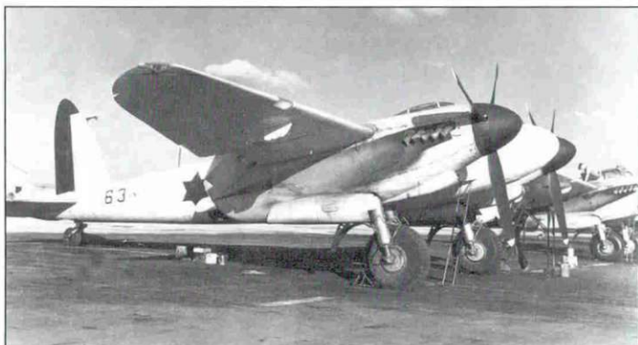
Above: The February 17, 1951 Mosquito purchase in France also included three TR Mk.33 conversion trainers. These aircraft were assigned to the Valley squadron and had an overall FS33637 Trainer Yellow finish with red spinners and rudder. In 1953 these TR Mk.33 trainers were transferred to the night fighter tactics evaluation unit and had their spinners and rudder painted black.
