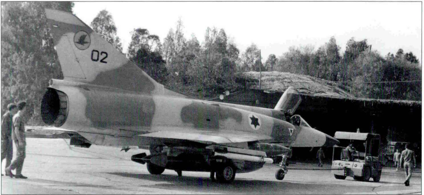
Above: Nesher no.02 of the Keepers of the Arava squadron accounted for 42 of the 277 Arab aircraft downed by the IAF during the 1973 Yom-Kippur War, with no loss to their own. The airplane is seen being towed to a hardened shelter carrying a pair of Shafrir II IR guided air to air missiles. The indigenously developed Shafrir II accounted for 120 of the air to air kills scored during the war. The Nesher (Eagle in Hebrew) was built in secrete by IAI using French "spare parts" and Atar 9C engine manufactured using drawings "stolen" from a Swiss engine manufacturer. Knowledge of the Nesher was considered secrete until its sale to Argentina in 1982.
