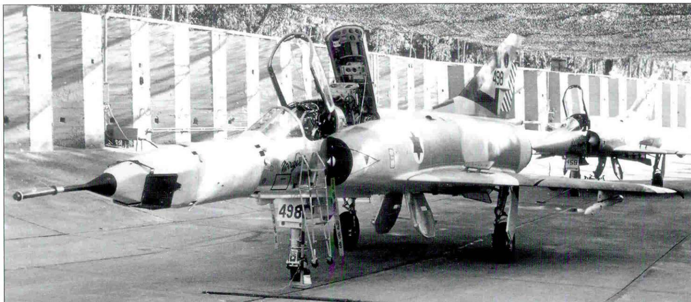
Above: The First Fighter squadron inherited the photo-recon roll from the Bat squadron when they transitioned to the F-4 Phantom prior to the Yom-Kippur War. Mirage no.498 is seen fitted with a long range side looking "Tzriot" recon camera and Mirage no.459 in the background is fitted with a "Moshel" look down recon camera. After the First Fighter squadron transitioned to the Kfir C2 in 1976 these nose sections were fitted to Kfir C2 numbers 419 and 451.
