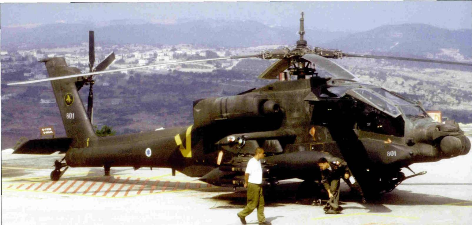
Top: AH-64A no.801 of the Hornet squadron is seen parked in a quick reaction alert configuration with two external fuel tanks, and eight AGM-114 Hellfire missiles under its stub wings. The 8XX series Apaches, named Peten (Viper) in Hebrew arrived in Israel on September 12, 1993 and entered into service with the Hornet squadron. The Apache retained its overall FS34031 black-green camouflage scheme well into 2005, until a new "Tiger Scheme" was applied to all 8XX and 9XX to all IAF Peten helicopters. Before the introduction of the AH-64D Apache Longbow "Saraf" to Hornet squadron service on April 10, 2005, all IAF AH-64A Petens were transferred to the Magic Touch squadron.
