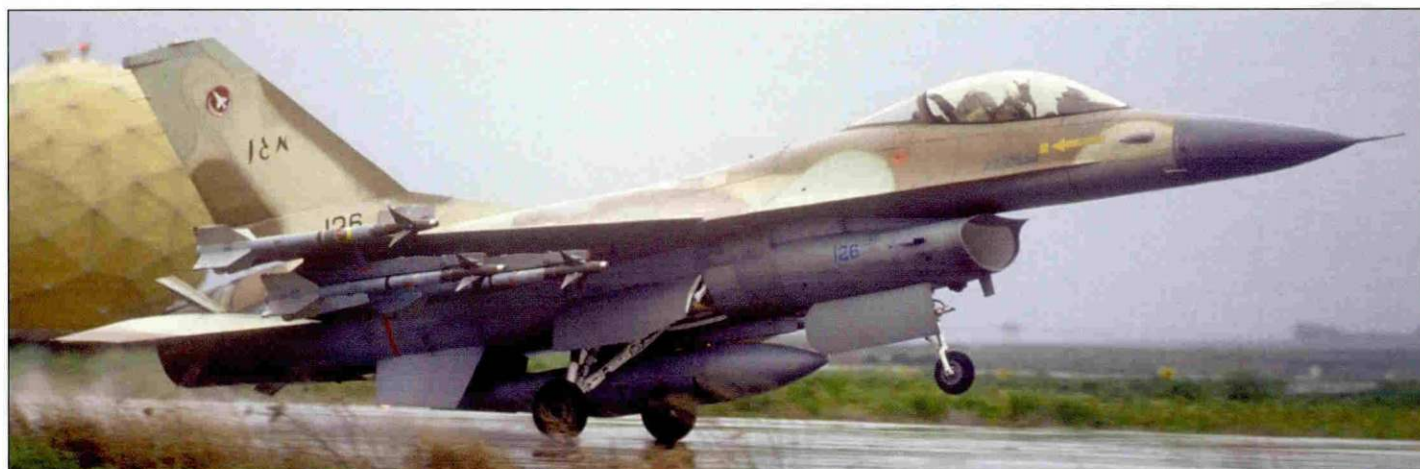
Above: F-16A no.126 "Magen" (Shield) of the First Jet Squadron is landing in an unusual configuration of six Sidewinders. In the Mid-'80's F-16A's of the First Jet and Knights of the North Squadrons were fitted with large horizontal stabilizers and external chaff/flare dispensers on the vertical fin root and between the aft fuselage ventral fins.
